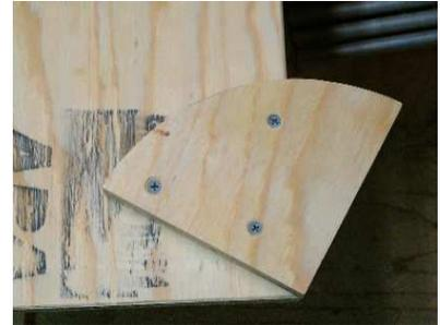
The key to the stability and economy of this system is the use of plywood disks on the bottom of the lid modules lock the lids in position on the buckets. No other hinges, locks, or latches are needed.
