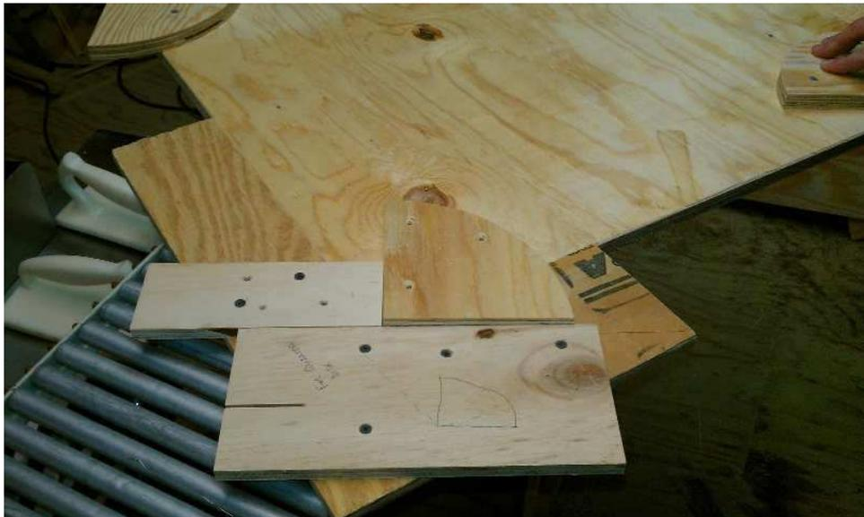
Similarly, the quarter disk jig is made of four pieces of ply, locating the center of the disk directly over the inside corner of the lid, with the radial sides of the quarter rotated 30 degrees CLOCKWISE from the edge of the lid. All partial disks are mounted 30 degrees CLOCKWISE.
