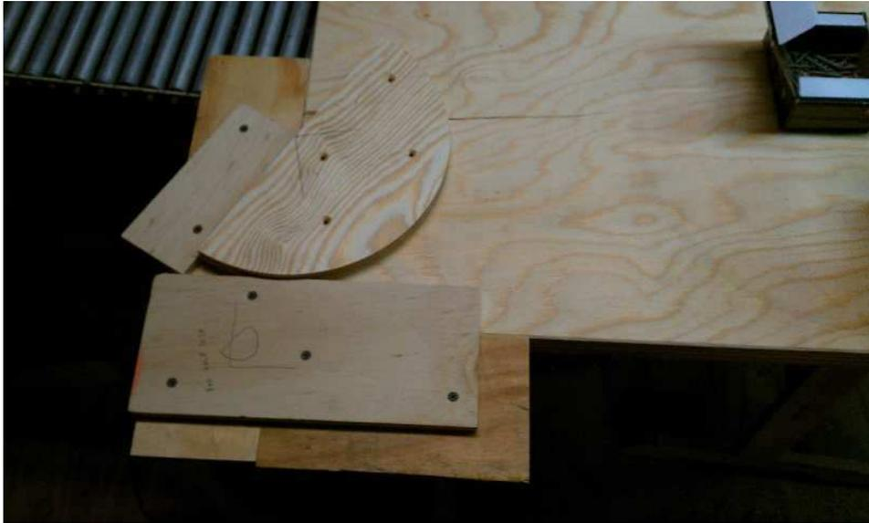
I screwed together four pieces of plywood to locate the edge of the half disks in 1.625 inches from the outside edges. In that position, they will clear the chair rail strips on nesting lids for storage. (and theoretically allow for double-stacking risers)
