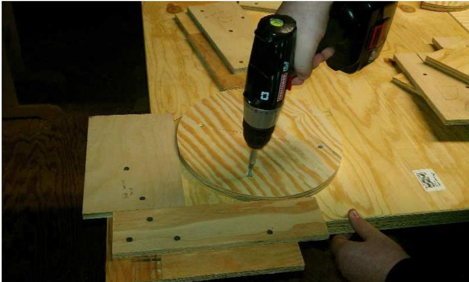
I screwed together four pieces of plywood to locate the whole disks in 1.625 inches from the outside edges. In that position, they will clear the chair rail strips on nesting lids for storage. (and theoretically allow for double-stacking risers)
